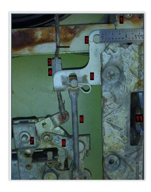
I could then remove the latch mechanism by removing the last two Phillips head bolts and clean it the same way. I then used a spray type automotive grease designed for latches and hinges to relubricate the mechanisms. For the key cylinder I used a dry lubricant made for this purpose.
